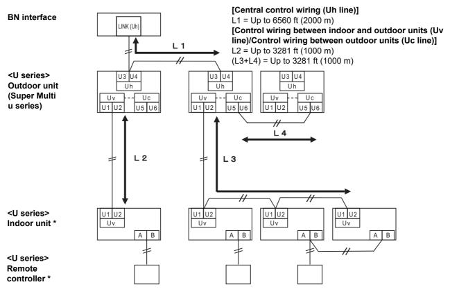
\* The wiring specifications in the system diagram above are the same even when the indoor unit or remote controller are other than the U series.
